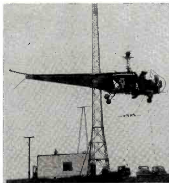
The helicopter with Mr. Robinson at the controls lifts the airborne antenna skyward for distortion tests.
